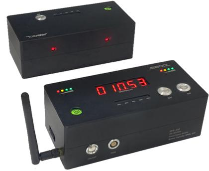
Speed Measurement Device SPS-5M, by two groups of high-speed laser sensors of front and rear installed in opposite direction, can detect the time difference of the object passing through the two sets of laser sensors. So that the speed can be calculated because the length is constant. The result can display by internal LED or external LED, and even remote PC.
