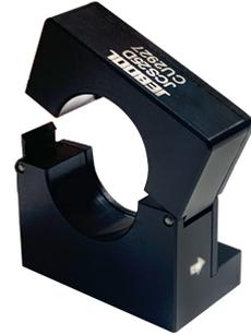
The current sensor JCS25D is based on the Hall principle to achieve high-precision measurement of line current. The independent power supply is completely isolated from the measurement system, and the direct output voltage signal has a good linear relationship with the measured current. JCS25D has default range 500A, and below 1000A is optional.
